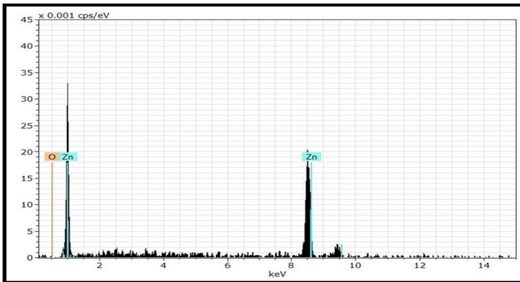
Figure (1): Shows the purity of zinc oxide nanoparticles using SDX device
