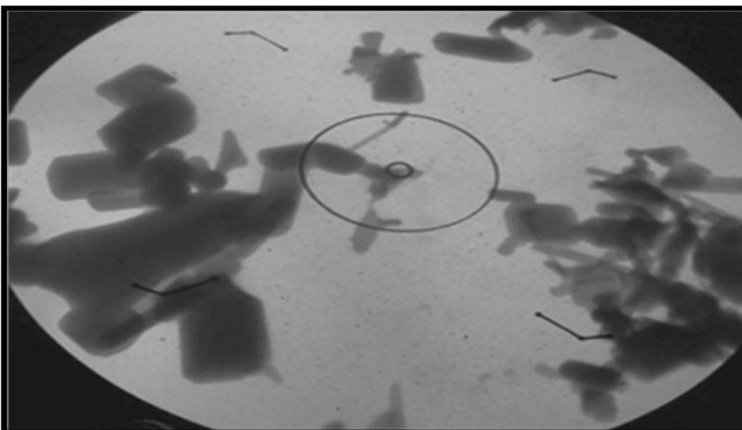
Figure (2): Shows the cubic shapes of zinc oxide nanoparticles using TEM microscope.
